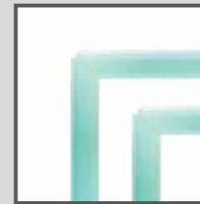
45° cut edges for front and top glass of showcase
